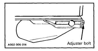
NOTE: Track tension and alignment are inter-related. Do not adjust one without checking the other.
