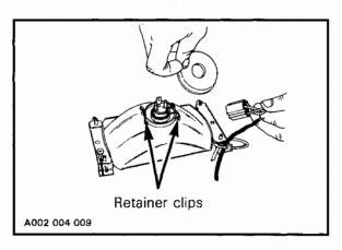
If taillight bulb is burnt, remove the red plastic lens and replace bulb.
