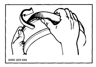
Slip the belt out from the drive pulley and remove completely from the vehicle. To install the drive belt, reverse the procedure, however pay attention to the following.
