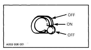
Ensure the tether cut-out cap is in position and that the cord is attached to your clothing.
