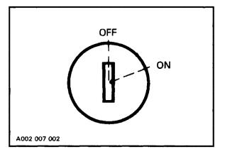
Key operated, two position switch. To start the engine, first turn the key to ON position. To stop the engine, turn the key to OFF position.
