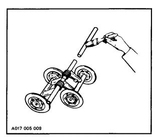
Grease each bogie wheel until the old grease is flushed out. Spray bogie wheel springs with metal protector. If unavailable, wipe with a cloth or rag soaked in oil.
