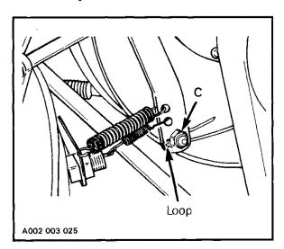
WARNING: Brake cable must make a loop around the bolt head. Strongly pull the brake handle to check cable tightness. Always check the brake light to see if it functions after performing brake adjustment.
