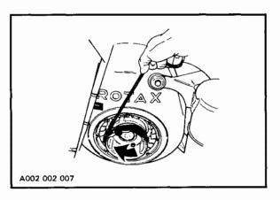
WARNING: After starting the vehicle in an emergency situation by the starting pulley do not reinstall the rewind starter assembly. When starting the vehicle in an emergency situation by the drive pulley, do not make a knot at the end of the emergency rope and do not reinstall the belt guard and pulley guard.
