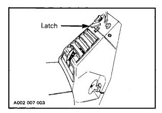
Push the console downward then tilt away from the engine. To reinstall, reverse the procedure.
