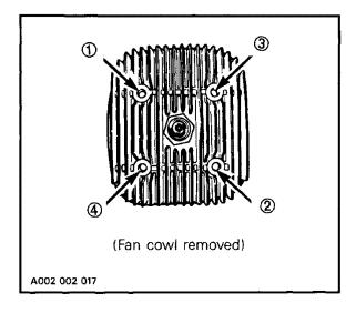
**IMPORTANT**: The engine head nut torque should be checked after the first five hours of operation.
