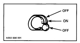
WARNING: For safety reasons, the emergency cut-off switch is easily accessible; be careful not to operate it inadvertently. If the switch has been used in an emergency situation, the source of malfunction should be determined and corrected before restarting the engine.
