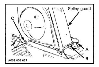
Push the pulley guard forward to disengage the front attachment (C) from the frame. Lift the guard from the vehicle.
