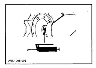
CAUTION: When lubricating the rear axle bearing, do not apply excessive grease as the seal will be pushed out of its housing. Check seal position with finger.
